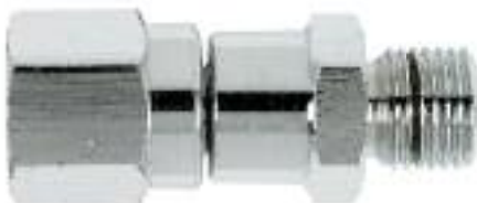
1235 G 1/4 Female with 60 cone seat & "O" Ring that swivels 360 degrees to G 1/4 Male stud. Only to be used in static conditions. e.g. behind a panel to line up valves etc. DO NOT use on charging hoses.
