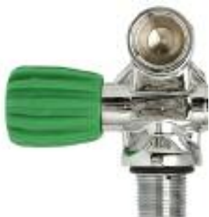
4000 NEW EUROPEAN NITROX VALVE. Regulator connection is 26 x 2 mm.
