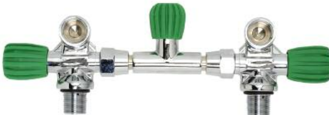
4065 NEW EUROPEAN NITROX TWIN MANIFOLD WITH CENTRE ISOLATION. M25 X 2 REGULATOR CONNECTION IS M26 X 2. AVAILABLE FOR ALL CENTRES. PLEASE SPECIFY.
