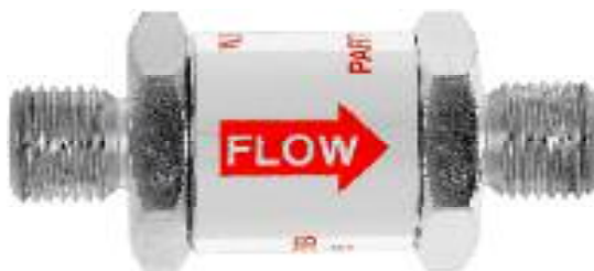
5100 One way valve with G 1/4 Male threads. Must only be used in static assemblies. Max W.P. 414 Bar.
