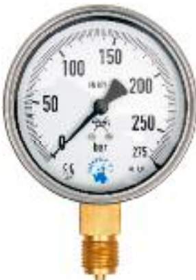
5098 0-275 Bar x 100 mm Dry for Oxygen use. G 1/2 thread. 1% accurate. Use our 1274 adaptor to convert to G 1/4. Scale now with 2 Bar increments.
