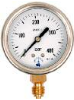
5090 0-400 Bar x 63 mm Oil filled for Air use only G 1/4 thread. 1.6%
