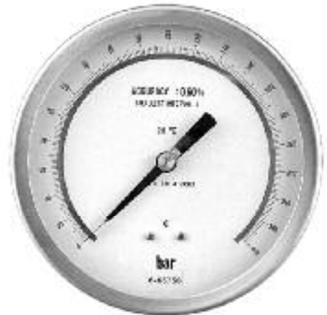
5080 150mm MIRROR SCALE GAUGE. 0—400 BAR Highly accurate to 0.6% of full scale. Adjusting screw on needle to re-zero. G 1/4 back connection for panel mounting with clamp supplied. Supplied with test certificate. Use our 1260 or 1272 gauge adapters for connecting.
